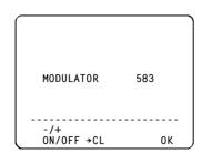
8 Switch the video recorder to standby with the STANDBY ර) button. **Note:** This modulator frequency (583MHz or UHF-channel 35) might already be being used by another TV station in your reception area, e.g. 'Channel 5'. In this case the picture quality on your TV set will be poor when receiving one or more TV channels.
